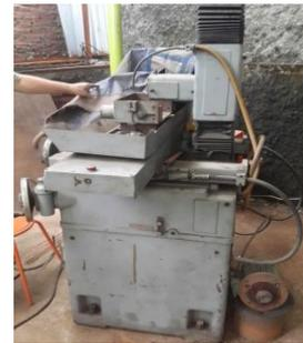
Gambar 4. Mesin Surface Grinding
